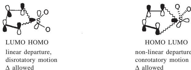
Figure 9. Frontier molecular orbital transition state analyses for cheletropic expulsion of \text{SO}_2 from sulfolenes.
