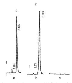
Figure 3. Representative chromatograms of (a) thymine standard, 1.6  $\mu$ g/mL (peak 1) and D4T standard 80.0  $\mu$ g/mL (peak 2); (b) D4T capsule sample 100.0  $\mu$ g/mL; (c) D4T capsule placebo
