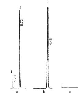
Figure 2. Representative chromatograms of (a) thymine standard, 1.5 µg/mL (peak 1) and AZT standard 90.0 µg/mL (peak 2); (b) AZT capsule sample 100.0 µg/mL; (c) AZT capsule placebo
