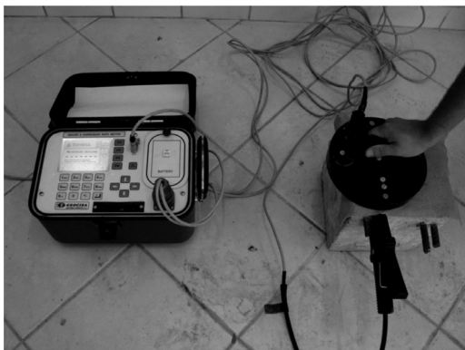
Figure 2. Measuring system to obtain the corrosion steel rate in a reinforced concrete sample
