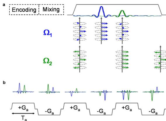
**Figure 2S.** (a) Representation of the ultrafast dimension acquisition by the application of a gradient pulse, in order to remove the dephasing created during the spatial encoding step. As result, the echo peaks are formed as the dephasing is being refocused. (b) Representation of the conventional dimension acquisition by the use of a bipolar pair of gradient pulses, which results in the monitoring of conventional parameters evolution as a series of sub-spectra are being collected
