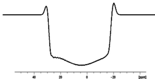
**Figure 3S.** Image of the excitation profile obtained from the pulse sequence in Figure 1 (with the extra block) and after phase correction, allowing for the chirp pulse power calibration before performing ultrafast experiments. The acquisition and processing parameters are the same mentioned for the Figure 2b, unless the chirp pulse power that was 0.32 W
