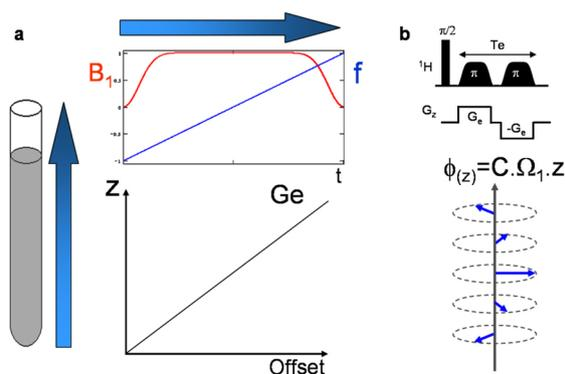
**Figure 1S.** (a) Graphical representation of continuous spatial encoding, in which a chirp pulse is applied concomitantly to a gradient pulse ( $G_e$ ) along  $z$  axis. (b) The scheme proposed by Pelupessy<sup>20</sup> comprises the application of a  $90^\circ$  hard pulse followed by two  $\pi$  chirp pulses applied together with a bipolar pair of gradients
